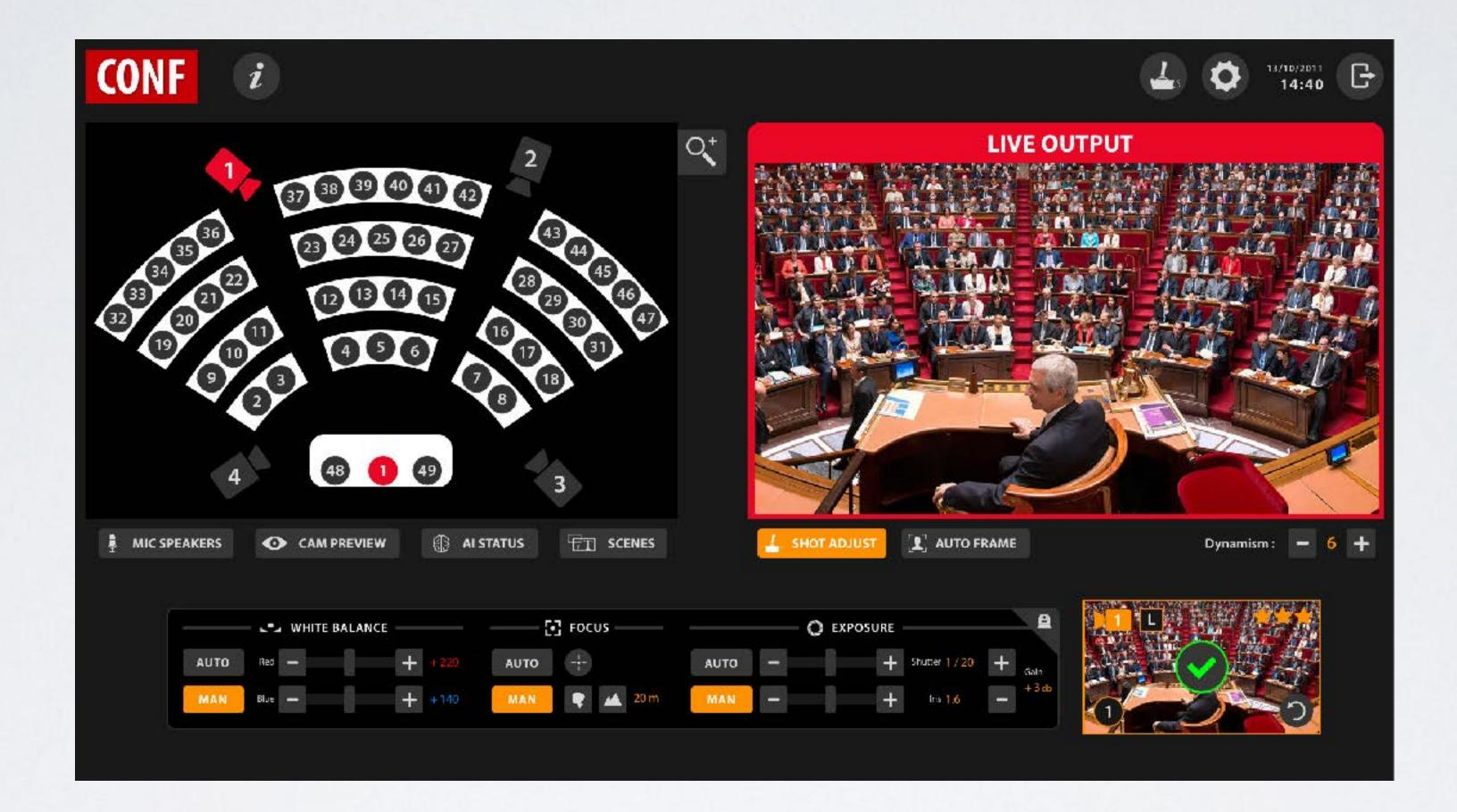
Each microphone is covered by different angles of shots with the PTZ cameras installed in the conference room.
